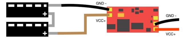
Optionally the two series connected capacitors can be replaced by two series connected 1 Farad / 2.7V capacitors for an increased storage time.
