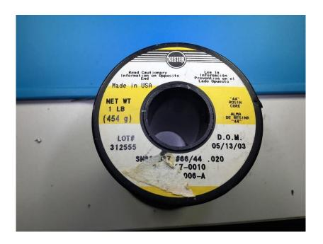
I use 60/40 lead solder. I like the 0.020" to 0.035" diameter Kester 44 solder for this work. The smaller the diameter the better.
