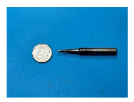
The Weller wlc100 40-watt soldering station with the original chisel tip and a Weller ST-7 soldering tip are enough to build an entire railroad and solder all your decoders if you are careful with the tips. Only the Weller tips hold up well. All can be found on eBay and elsewhere. It doesn't have to be this soldering iron. A 40 watt adjustable soldering iron with a fine tip for electronics and a chisel tip for track is what I recommend.
