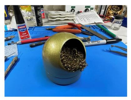
I use a brass ball to clean the tip of the soldering iron. It is the current and very effective way to preserve soldering iron tips.
